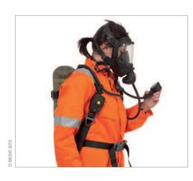
Close cylinder valve and breathe gently to exhaust air from system. Observe gauge, whistle will alarm at between 60 bar to 50 bar. Continue breathing down the system. Once empty, hold breath for approximately 3-5 seconds – the facemask should collapse and hold to face indicating a positive seal.
