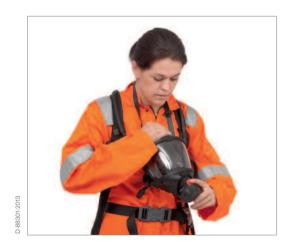
Reset lung demand valve by pressing red button in, taking care not to press centre of rubber cover.
