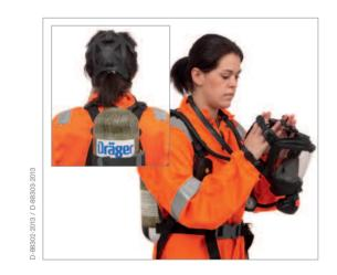
Unhook facemask from button, spread head harness and place over head with centre plate to the back. Place chin in facemask chin cup, tighten lower straps first then upper straps (holding breath). Tighten centre strap if necessary.
