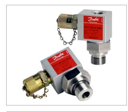
The MBV 3000 test valve is designed for test of the Danfoss cartridge pressure transmitters within the marine industry. The main advantage is the ability to test the operating transmitter through the test connection. A built-in shut-off valve gives the possibility to maintain transmitter without having to drain the system. After the transmitter is tested, the valve is manually re-opened and the transmitter is again connected to the system.
