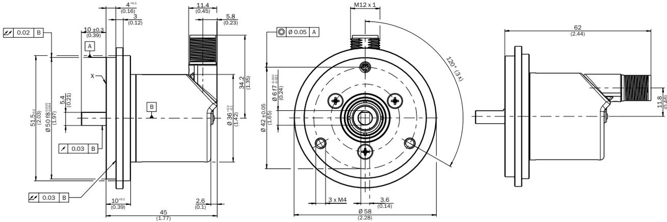
X = Measuring point for operating temperature
