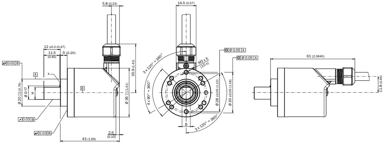
X = Measuring point for operating temperature
