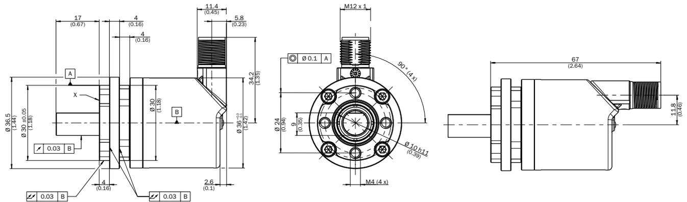
X = Measuring point for operating temperature
