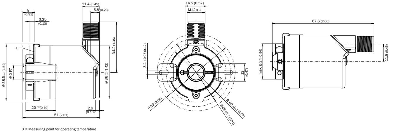
Customer-side shaft: Insertion depth min.15 mm ... max 22 mm, from contact surface stator coupling, recommended shaft-fitting: k7
