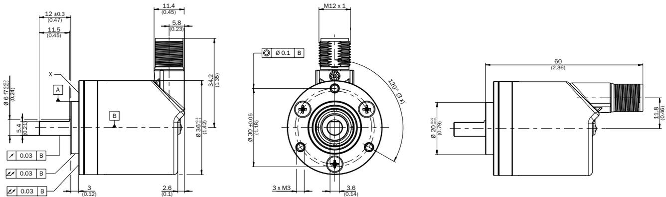
X = Measuring point for operating temperature
