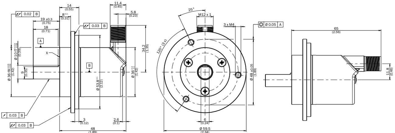
X = Measuring point for operating temperature
