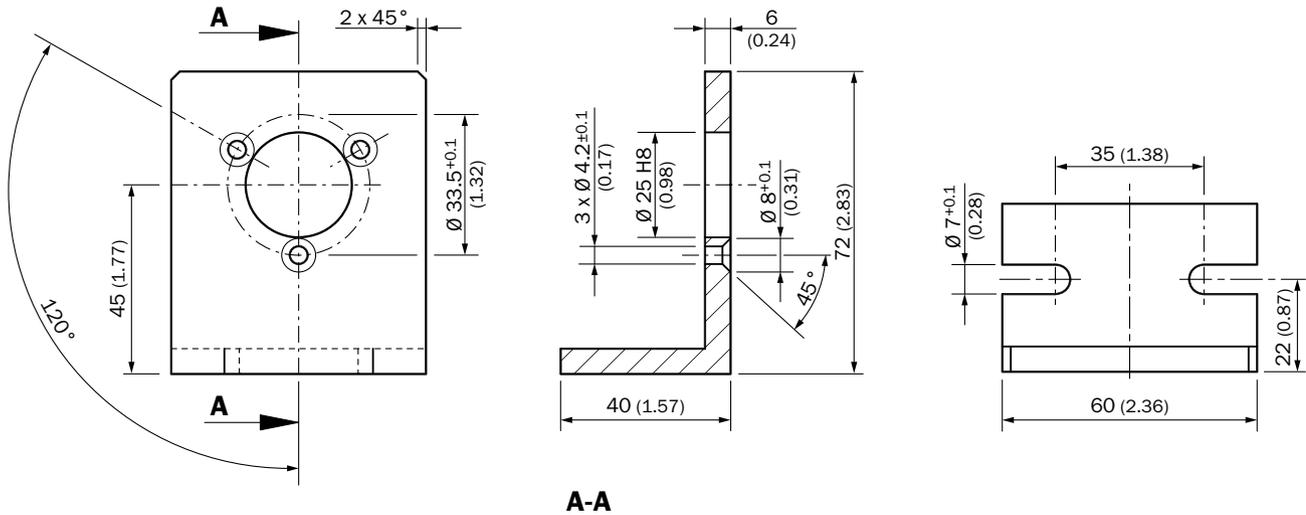
Dimensional drawings for mounting systems, flange
