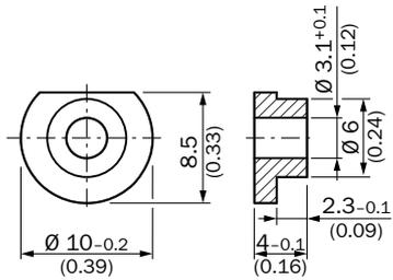
Dimensional drawings for mounting systems, shaft adaptation
