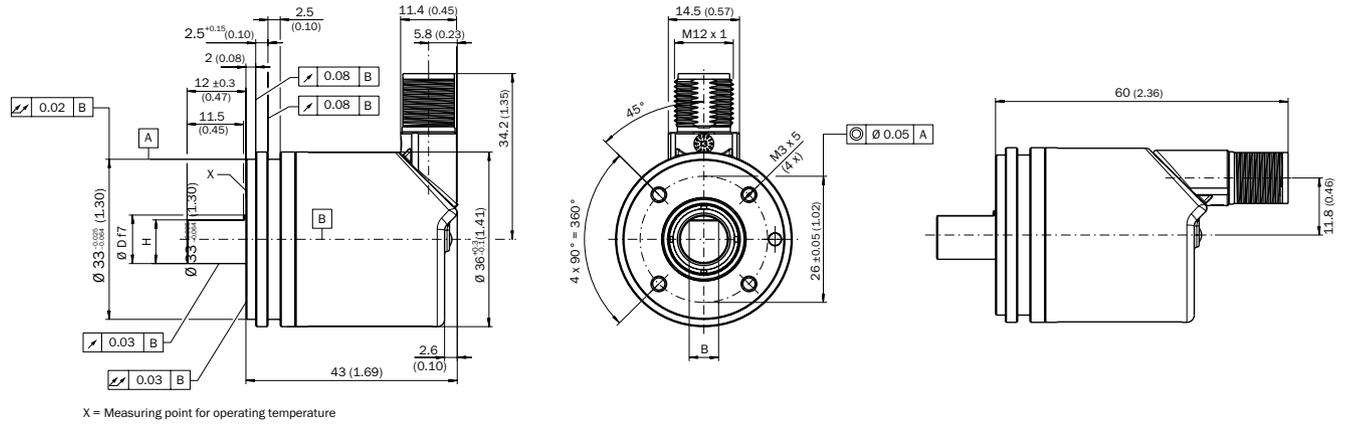
Solid shaft, servo flange, cable output
