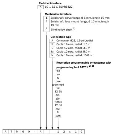
$<sup>^{1)}</sup>$  Collets for 6, 8, 10, 12, 14 mm and 1/4", 3/8" 1/2" as accessories, seperate order item (see recommended accessories). For 15 mm shaft diameter collet is not needed.
