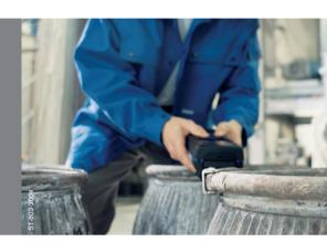
Two components define the system: the Analyzer and the substance-specific chip.
