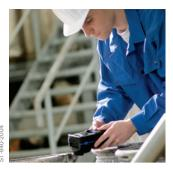
**Dräger CMS**Spot measurement at industrial workplaces
