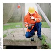
Dräger CMS with Remote-System Measurement with extension hoses of up to 10 m in length
