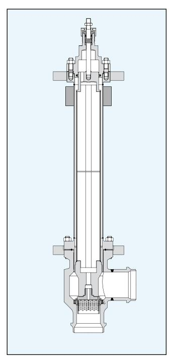
Low temperature valve with pressure balancing and multi-hole cage plug
