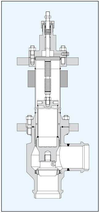
Low temperature valve with bellows seal and test connection
