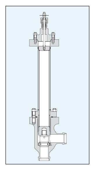
Control valve model 041500 for air separation. Aluminium body with and stainless steel extension for "Cold-Box" systems. On sizes DN 25 / 1″ to DN 100 / 4″ the trim can
