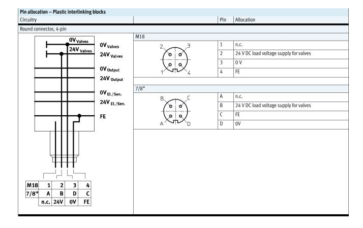
Accessories – Interlinking block with additional power supply for valves
