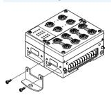
For longer valve terminals, there are additional mounting brackets for the CPX terminal that can be screwed onto the interlinking blocks.
