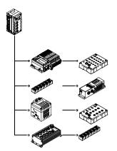
The CPX-CP electrical interface establishes the connection to CP modules of the CPI installation system via prefabricated connecting cables. The I/O data of the connected valve terminals with CP string extension and CP input and output modules are transferred to the connected CPX bus node and thus via fieldbus to the higher-order controller.
