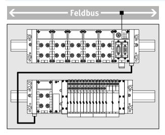
The extension enables the CPX terminal to be separated into or configured as two interconnected units (series).
