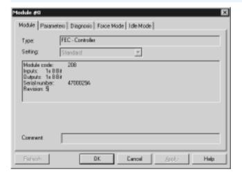
Displays important module data as well as the number of allocated inputs and outputs.
