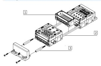
The CPX modules are mechanically connected using special tie rods 2. Two screws in the end plates are all that are needed to assemble the entire unit.
