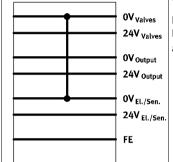
The module combines the 0 V potential of the power supply for electronics and sensors with the 0 V potential of the power supply for valves.
