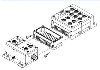
The CPX modules are mechanically connected using a special angled fitting.
