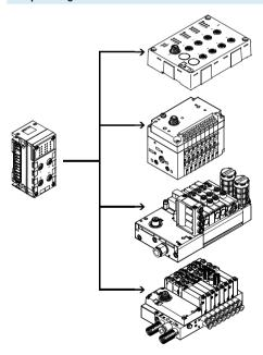
The CPX-CTEL master provides four I-Port interfaces to which one device each can be connected. I-Port is an interface for exchanging serial data for connecting decentralised modules or valve terminals from Festo. The I-Port interface is based on IO-Link and is compatible with it in certain areas.
