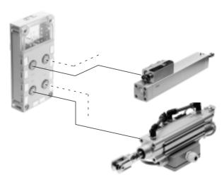
Since the module supports the M12 connection block (8-pin), up to 4 cylinder/valve combinations with integrated sensors can be connected. Each cylinder/valve combination is supported by 2 inputs and 2 outputs per connection. It is therefore possible to control max. 2 solenoid coils and record signals from 2 sensors with a pre-assembled connecting cable.
