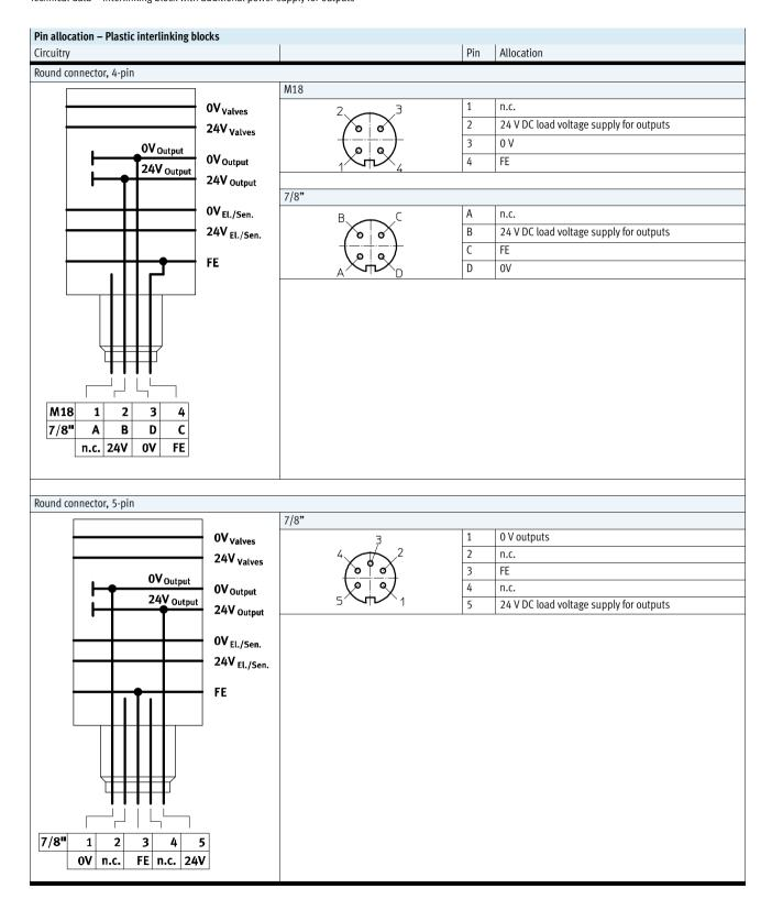
Technical data – Interlinking block with additional power supply for outputs
