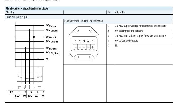
Accessories – Interlinking block with system supply
