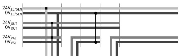
The use of decentralised devices on the fieldbus – particularly with a high degree protection for direct machine mounting – demands a flexible power supply concept. A valve terminal with CPX can, in principle, supply all voltages via a single connection. A distinction is made between the supply forElectronics plus sensors
