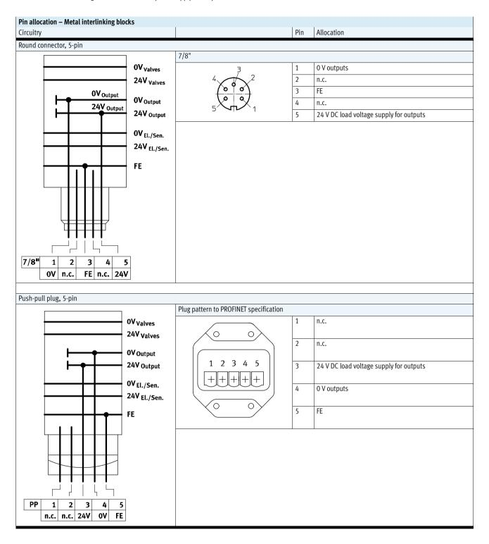
Accessories – Interlinking block with additional power supply for outputs
