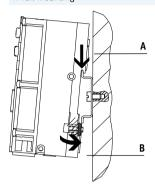
The H-rail mounting is part of the reverse profile of the CPX interlinking blocks. The CPX terminal can be attached to the H-rail using the H-rail mounting kit.
