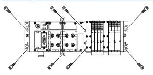
The end plates of the CPX terminal, the valve terminal and the pneumatic interface include mounting holes for wall mounting. Additional mountings for the CPX terminal are available for longer valve terminals. These mountings differ depending on the design of the CPX terminal (plastic or metal).
