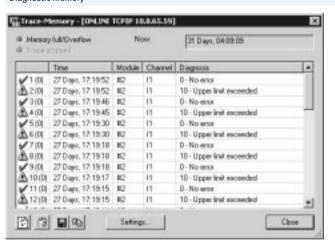
Faults which occur during operation are entered in a diagnostic memory. The first or the last 40 entries are saved, as well as the respective time measured from the moment the power supply was switched on.
