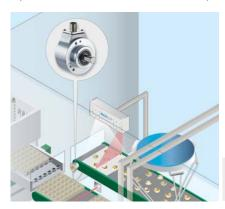
The DBS60 Core incremental encoder measures the speed of the belt. Pralines of different types are transported on the belt and sorted into the trays with a Pick & Place robot. The processes must be synchronized and the encoder provides the required process speed.
