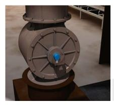
Rotary valves control the carbon and sinter supply for the subsequent processing steps. The ATM60 PROFIBUS absolute encoder provides information about the position of the valve which is used to control the amount and speed of carbon and sinter when they are supplied to the subsequent processes. Their magnetic scanning system makes these encoders ideal for use in harsh environments.
