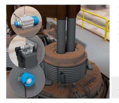
Cylinders and motors raise or lower the cover of the ladle furnace depending on the process step. Certain processes can only be performed safely if the ladle furnace cover is in a particular position. An absolute or wire draw encoder monitors the movements and positions
