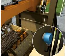
The height of the hold-down arm is detected with the ATM60 position encoder for determining the log diameter. The rotation time is calculated from this.
