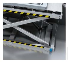
Following machining, residual grids are placed on a scissor lift table. To ensure a smooth transfer, the height of the stack must be aligned with that of the machining table. The analog signal values of the EcoLine wire draw encoder are used to determine the lifting height. When the maximum load has been reached, the worker removes the stack of residual grids.
