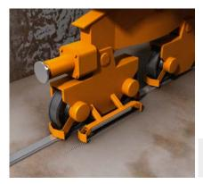
A non-contact KH53 linear encoder with a resolution of 0.1 mm and optionally for measurement lengths up to 38, 107, 354, and 1700 m is used for detecting
