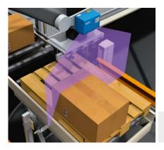
With both laser measurement and absolute encoders, an image and a position of the load can be determined, enabling the robot system to accurately pick up and transfer the material.
