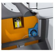
The BCG08 EcoLine wire draw encoder determines the fork lifting height of the automated guided system and forwards this to the vehicle controller.
