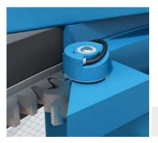
After the pallet has reached its position, the stretch film is secured to the pallet and wrapped using upward and downward movements of the film. The number of windings is determined via a gear wheel on the sprocket with an AFM60 absolute encoder.
