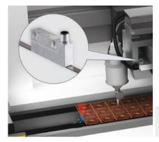
Semiconductor chips are placed in bonding machines at high speed, which assumes the greatest precision. The non-contact TTK70 linear encoder works with a precision in the  $\mu$ m range, thus enabling the precise positioning on the lead frames.
