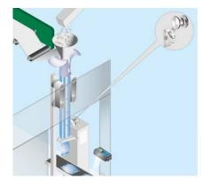
The DBS50 Core incremental encoder monitors the speed of the packaging film on a bag packaging machine. This measurement is required in order to control the fill quantity and cutting process. For slip-free speed measurement, an alternative is to use the DFV60 incremental measuring wheel encoder.
