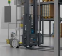
Positioning of the forks of the AGS is handled by constantly-measuring wire draw encoders. This way, the bays are approached at the correct height.
