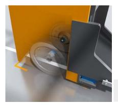
The route of the automated guided system (AGS) is stipulated by the higher-level control system. The DFS60 incremental encoder determines the speed of the wheels of the AGS. This information is used to control the warning fields of the safety laser scanners.
