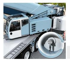
The angle and the position of the boom relative to the lower carriage must be known for a stable load torque restriction. The AHS/AHM 36 absolute encoder
