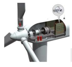
Generally, incremental encoders are used to monitor the rotor speed. These are normally fastened to the hub of the rotor. The DFS60 incremental encoder is used around the world under the harshest conditions. Its stable construction with enclosure rating up to IP67 makes it a robust and nevertheless
