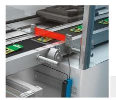
The DBS60 incremental encoder transfers the position of the belt for synchronization of both sensor signals. Alternatively, the belt speed can be taken directly on the belt using a measuring wheel encoder. This can reduce slippage.
