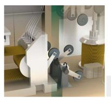
The precise use of saw-wires assumes the use of appropriate encoders. With the AFM60 absolute encoders from SICK, damage to wafers is minimized. The absolute encoders check the precise position of the saw-wire and transmit the data with the resolution required for this process.
