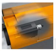
The DBS36 Core incremental encoder or the AHM36 absolute encoder supplies the value for controlling the positioning, speed, and acceleration. The encoder ensures that the positioning of the shuttle can be executed with precision. The DFS60S Pro can help to realize these safety functions.
