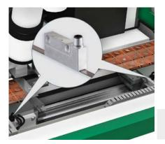
Temperatures are very high in the area around the bonding head, making fiber-optic cable systems the most effective for this application. With its 16 µs response time, the WLL180T works together with the LL3-TH fibers to supply the control unit with a precise signal for edge detection. The grippers of the wire
