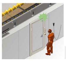
On the saw line, the operator is kept away from the hazardous point by a safety fence. In order to eliminate faults on the line, a safe standstill detection is necessary or for the maintenance and service mode, a safely-limited speed. The DFS60S Pro safety encoders assist reliably with the realization of safety functions.
