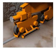
A rugged linear encoder can be used for precise positioning. The KH53 non-contact, virtually maintenance-free linear encoder is installed on the crane column to ensure that the X-axis of the crane is detected correctly. The encoder detects the absolute crane position by detecting the integrated magnets which are installed parallel to the crane rails.
