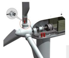
The adjustment of the rotor blades plays an important role in order to achieve as great a yield as possible of rotation energy. Depending on the wind strength and direction, the position of the rotor blades is adjusted accordingly. AFS60/AFM60 absolute encoders are used to set the rotor blades.
