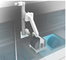
The position of the wafer carrier is determined reliably with absolute encoders: with the AFS60 Singleturn on the vertical and the AFM60 Multiturn on the horizontal axis. Thanks to SSI and industrial Ethernet interfaces, it is possible to integrate these into the machine controller easily and cost-effectively.
