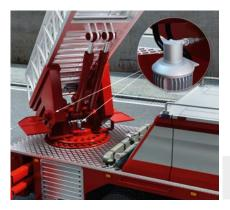
The angle and the position of the aerial ladder relative to the lower carriage must be known in order to carry out repeating movement sequences. The absolute encoders from the AHS/AHM36 product family are the right sensor solution thanks to their compact and rugged design and high repeatability.
