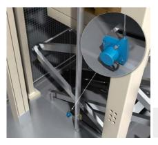
The scissor lift table is positioned using a high-resolution wire draw encoder with a teach-in function. The extremely reliable wire draw encoder does not require complex linear guidance, and can be integrated with ease both electrically and mechanically.
