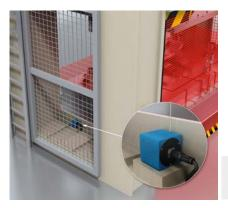
To determine the position of the press stroke, a BKS wire draw encoder is used. It reliably supplies signals for
