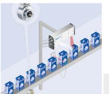
The DBS60 Core incremental encoder measures the speed of the belt. This information is required in order to control
