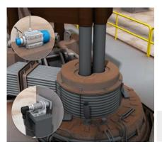
Electrode arms raise and lower the electrodes of a ladle furnace. In some cases, the position of the electrodes is crucial for other movements or for the timing of subsequent process steps such as the movement of the ladle. To ensure safe operation of a ladle furnace and to op-
