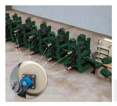
Synchronization of rollers and their stands during the hot rolling process is important in order to ensure consistent product quality. Production optimization is also attained via proper control of the rolling stands. Absolute and incremental encoders regulate the drive motors of the rolling stands during the hot rolling
