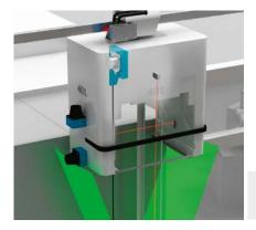
The risk of material breaks in expensive semiconductor wafers must be kept as small as possible. Therefore, the wafer box is monitored with sensors. The Ecoline product family of wire draw encoders – lightweights at just 180 grams – provide the exact position of the FOUPs (wafer box) during lowering.
