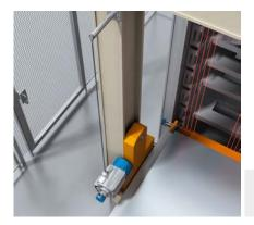
The material lift is used to move stacks of sheets from a transfer carriage or residual sheets from a vacuum nozzle to an interim shelf for storage. The BTF13 wire draw encoder signals the absolute height position of the material lift to the control. The bottom and top final positions of the material lift are monitored by inductive proximity sensors.
