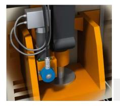
Once the tools have been replaced, the press stroke must be adapted using a primarily mechanical adjustment mechanism. The procedure for adjusting the height of the press stroke can be done
