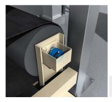
The conveyor belt speed at which the bio mass is transported to the shredder and then to the storage location is very important when it comes to controlling the material flow. The DFS60 incremental encoder calculates the speed and running direction of the belt. The DFS60 encoder can be configured either via a PC or with a separate programming tool, thus offering comprehensive programming flexibility for all industrial requirements.
