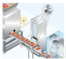
The DBS60 Core incremental encoder is used to regulate the speed of the belt. Both belts must be speed-synchronized
