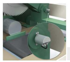
The height of the saw blade is automatically positioned for optimum control of the sawing process. The DBS36 Core incremental encoder supplies precise measurement values for this purpose. It can be easily and directly mounted using the face mount flange or the hollow shaft and its universal cable outlet. Its compact size saves space.
