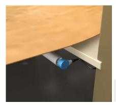
The length of the veneer material is measured precisely with the ATM69 absolute
