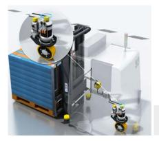
With automated guided systems (AGS), the SSM (safety speed monitor) or SLS (safety-limited speed) function monitors the speed on the wheels using the DFS60S Pro encoder and reduces it via the controller if necessary. Thanks to a central drive unit, with the DFS60S Pro and the Flexi Soft safety controller, it is possible to realize safe motion monitoring or warning field monitoring of the safety laser scanner.
