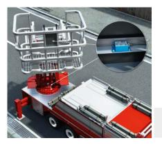
In order to transport people smoothly and horizontally, the TMM61 two-dimensional inclination sensor determines the inclination of the cage and sends this information to the higher-level control for regulation purposes. With its compensated cross sensitivity and configurable vibration suppression, the TMM61 enables precise, reliable positioning.
