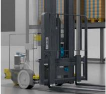
The measurement of the fork lifting height on the AGS for the precise removal of print products from the
