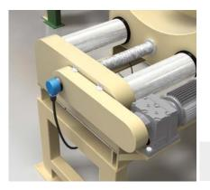
The positioning of saw-blades for setting to the thickness to be sawed is done with the ATM60 absolute encoder.
