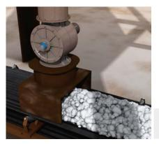
Although rotary valves are small parts in big steel plants, they play an important role in the material flow process which is vital for uninterrupted steel making. Typical locations for rotary valves include discharging positions for bulk materials, dust or ash from silos, bunkers and hoppers or transfer points in conveying systems. To ensure proper functioning of all system parts, encoders monitor the valve on the basis of the axle movement.
