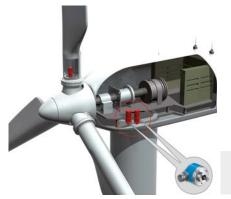
Depending on the change of the wind, the gondola must be aligned in the optimal wind direction. Thanks to the ATM60 absolute encoder, the correct rotation and function of the system is monitored, since precisely with strong winds there are very high forces and a malfunction of the gondola controller can result in high costs and downtimes.
