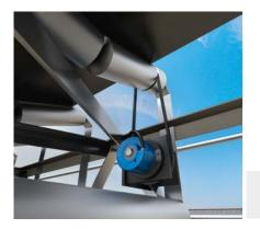
The belt speed at which mined materials are transported to stockpiles, ship loaders, and railroad loading facilities is of paramount importance. The DFS60 incremental encoder precisely calculates the speed and running direction of a belt. The DFS60 encoder can be configured either via a PC or with a separate programming tool, thus offering comprehensive programming flexibility for all mining requirements.
