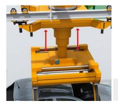
The electrical overhead conveyor brings the car bodies to designated workplaces. The compact BCG wire draw encoder ensures that the defined height position
