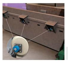
DFS60 incremental encoders monitor the motor of a rolling stand and therefore also the speed of the rolling mill train which transports the steel rods. Monitoring the train's speed helps to ensure product quality and to optimize the rolling process. The advantages of an in-
