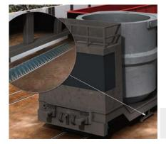
Proper positioning of outdoor rail-mounted shuttles during the material handling process is simple with the help of a linear encoder. The measuring element of the encoder is set in concrete between the rails. The encoder itself is mounted underneath the moving shuttle. This precise, non-contact positioning system identifies all shuttle positions on the rail. The rails do not need to be straight. The linear encoder can also handle elongated curves.
