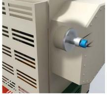
An ATM60 absolute encoder is mounted to the eccentric shaft on mechanical presses for the purpose of determining the position of the press stroke.
