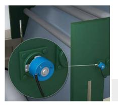
The DBS60 incremental encoder monitors the speed of the film sheet on a roller. This enables the film sheet to be wound up onto the coil at a constant rate.
