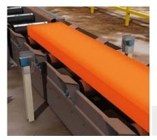
Positioning the cutting torch during the continuous casting process is an important step in guaranteeing that each object is precisely cut to length. DFS60 incremental encoders enable accurate positioning of the cutting torch once the liquid steel has been cast. The encoders feature a metal code disc with high temperature resistance – an undeniable requirement for use in a continuous casting plant.
