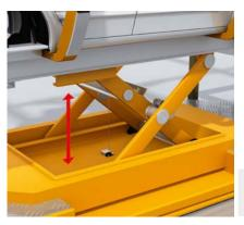
The compact BKS wire draw encoder measures the height of the scissor lift table accurately and forwards this to the controller of the scissor lift table via the SSI interface.
