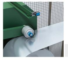
To ensure a constant feed of material, the uncoiling speed of the sheet coil must be regulated. The distance sensor continuously measures the radius of the sheet coil throughout the entire unwinding process. The DBS60 Core incremental encoder uses a friction
