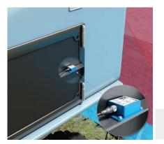
The TMS/TMM88 inclination sensor is used for reliable leveling of the driver's cab. Thanks to its efficient filter algorithms to suppress vibrations and its rugged design, it is particularly well suited for use in harsh ambient conditions. Its high accuracy over the entire measuring range and its outstanding temperature stability offer further advantages in such conditions.
