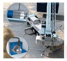
A sub-function for the load torque restriction on the mobile crane is the position detection of the extendable support feet and the detection of the boom and crane arm position. The wire draw encoders from the EcoLine product family are
