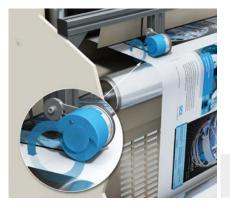
Certain digital printing machines fire individual ink droplets onto the paper per drop-on-demand and with the highest accuracy. The DFS60 incremental encoder uses a measuring wheel to detect the
