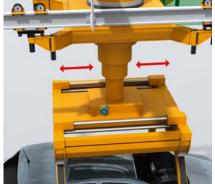
The electrical overhead conveyor brings the car bodies to designated workplaces. The speed is specified by the higher-level control; an incremental encoder deterIn case of requirements for secure speed, the DFS60S Pro assists with the realization of collision protection in combination with a safety laser scanner.
