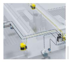
The movements of the CNC portal, which the worker cannot predict and which can be very rapid, represent hazardous points during the machining process. The modules of the Drive Monitor FX3-MOC safely monitor the electric drive system of the CNC plasma cutting machine in conjunction with the signals of
