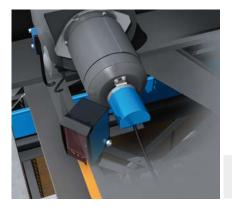
The shuttle is positioned by means of an incremental encoder mounted on the drive axis. Designs featuring a blind hollow shaft or a face mount flange with a solid shaft ensure flexible adaptation to the drive. They can even be used in cases where there is very little space available. Alternatively, an absolute encoder can also be used.
