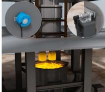
The vacuum chamber of a Ruhrstahl-Heraeus degasser is raised and lowered depending on the process step and fill level of the ladle. The lower part of the vacuum chamber dips into the liquid
