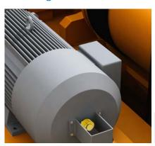
The information for the safe speed and direction of rotation monitoring of the crane winch is generated by the DFS60S Pro safety encoder. This way, hazards due to excessive speed or acceleration can be prevented depending on the cargo.
