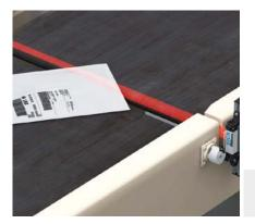
The leading edge detection serves to convey objects at a specified distance from the belts to the main sorter. The combination of high-resolution light grids and high-resolution encoders allows leading edge detection and the detection of additional object profile information such as the length.
