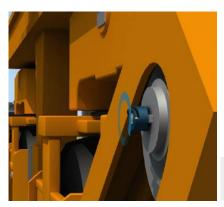
The speed of the drive motor of a crane is measured with the DBS60 incremental encoder. This way, the speed can be controlled depending on the cargo and the travel path of the crane determined.
