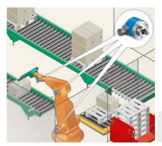
ATM60 Multiturn absolute encoders transmit the absolute positions of the
