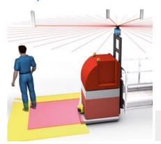
For personal protection and collision prevention with other vehicles or materials on the floor, automated guided systems AGS are equipped on the fork side and on the back wide with safety laser scanners. The AGS is equipped with two drive units with one DBS60 Core incremental
