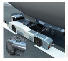
It is important to check the exact position of the nose wheel receptacle flap in the nose wheel receptacle. The singleturn version of the AHS/AHM36 absolute encoder is used for this purpose. It can also be used in harsh ambient conditions thanks to its rugged and reliable, fully magnetic sensor technology. Thanks to its small size, the encoder fits into even restricted installation spaces.
