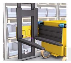
Using a BKS09 wire draw encoder enables the narrow aisle truck to accurately determine the position of the fork. The highly flexible steel wire is fixed to the fork's 'shoulder'. The driver sees the position of the fork on a display. This provides support when the height of the fork cannot be seen (man-below system).
