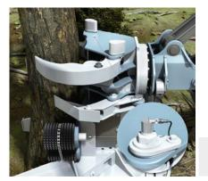
The rugged and highly compact AHS/ AHM 36 absolute encoders determine the gripper position to measure the treetrunk diameter. A further encoder determines the feed rate, thereby measuring the length of the trunk.
