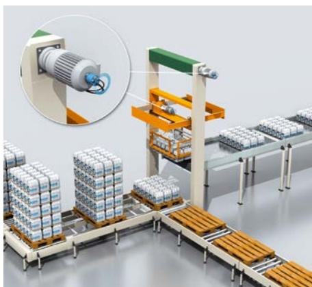
Palletizer system – positioning the gripper
