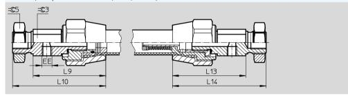
$MAS-...-EA/BA-EG/BG-pneumatic connection, \ radial, \ with \ threaded \ rod, \ one \ end/both \ ends$
