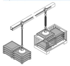
Achieving intermediate positions? Very simple, using pressure regulation: the workpieces can be raised or lowered as required by pressurising or exhausting the muscle via a hand lever valve. Muscle lengths up to 9 m facilitate various types of application.
