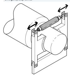
The Fluidic Muscle is setting benchmarks in applications that require fast response times. The emergency stop for rollers demands both speed and a high initial force. This can prevent risks to the operator in the event of malfunctions.
