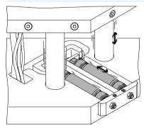
In joining processes such as those that take place in welding machines, the components to be welded are held in place by the Fluidic Muscle during the joining procedure. Here, too, the muscle can make the most of its high force combined with a small diameter.
