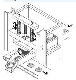
Very high cycle rates can be achieved with the muscle, on the one hand because of its low weight and on the other because it has no moving parts (e.g. a piston). The simple design – one muscle pretensioned using two springs – replaces a complicated toggle lever clamping system using cylinders.
