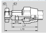
$MAS-...-ER/BR-EG/BG-pneumatic connection, \ radial, \ with \ threaded \ rod, \ one \ end/both \ ends$
