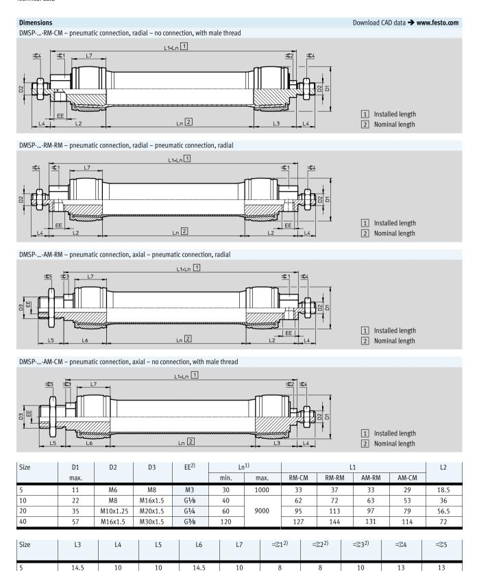
1) Tolerance < 100 mm ±1 mm, 100 ... 400 mm ±1%, > 400 mm ±4 mm.
