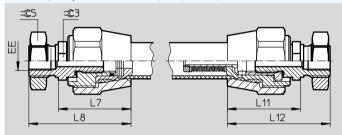
MAS-...-ER/BR – pneumatic connection, radial, one end/both ends
