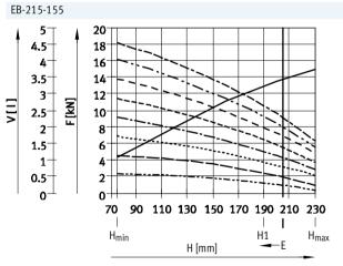
E Preferred range of application: Outside this range, the force reduces to a level so that the use of the next largest size is recommended.
