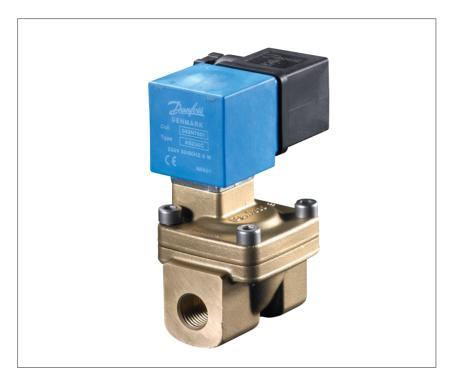
EV220W is a range of compact indirect servo-operated 2/2 way solenoid valves, especially designed for water inlet, with EPDM seal and WRAS approval.
