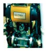
and top-mount actuator bracket design, this ball valve is very durable and can handle pressures to 5000 psi and temperatures to 450°F.
