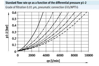
Grade of filtration 0.01 µm, pneumatic connection G1/NPT1
