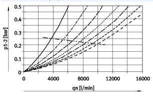
Grade of filtration 0.01  $\mu m$ , pneumatic connection G11/2/NPT11/2
