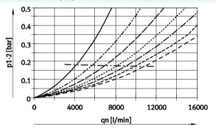
Standard flow rate qn as a function of the differential pressure p1-2
