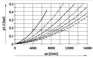
Grade of filtration 1  $\mu$ m, pneumatic connection G1<sup>1</sup>/<sub>2</sub>/NPT1<sup>1</sup>/<sub>2</sub>
