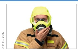
Check the fit of the half mask by closing the front filter opening with the palm of your hand. If negative pressure is not generated, readjust the half mask to ensure a close fit.
