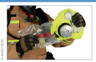
Hold the foil pouch on the bottom end firmly together with the red tear-away straps and at the same time pull the fire escape hood out until the filter plugs are completely removed from the filter.
