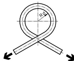
The tube is bent in the direction of its own curve until the tubing outer diameter is flattened by 5%.  $R_d$  is then calculated mathematically. The flow rate is not reduced until  $R_d$  is reached.
