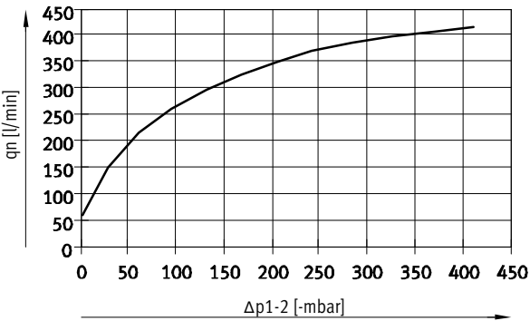
Standard flow rate q_n as a function of differential pressure \Delta p_{1-2}
