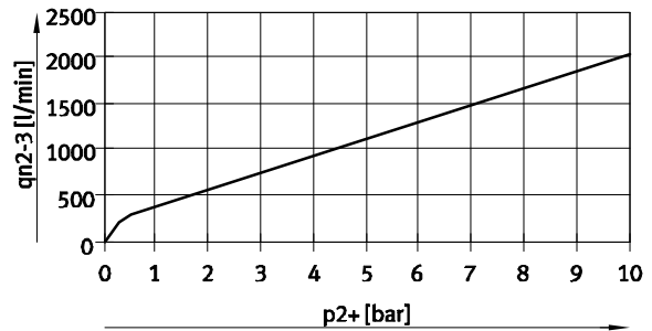
Flow rate q_n from 2 \rightarrow 3 as a function of output pressure p_2
