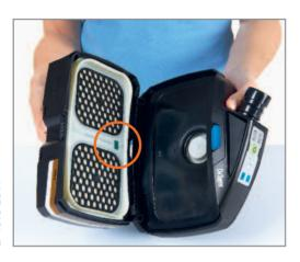
Gas / Combination filter I: Insert the filter (with the colour marking pointing downward towards the device) at an angle into the unit.
