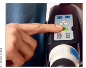
Press the green button on the control panel. The device performs a self-test.
