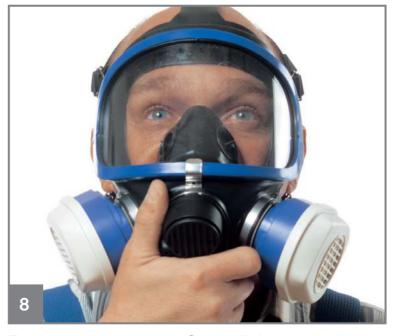
Positve pressure test: Seal off the protective cap of the exhalation valve with your palm and exhale. The mask will inflate slightly. If the mask does not inflate slightly, readjust the face piece and adjust headstraps or use a different mask size. Repeat the test until a successful fit check is met.
