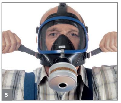
Tighten straps until the mask fits snug and secure. First tighen both neck straps, ...
