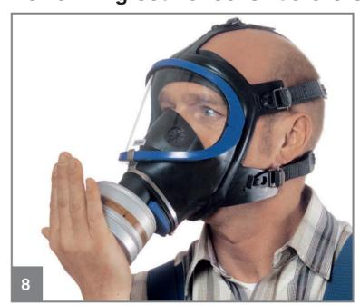
Negative pressure test: Seal respiratory filters with your palm and breathe in until a negative pressure (suction) is generated. Hold your breath for a mo-ment. The negative pressure should be maintained. If not, readjust the face piece and adjust the straps. Repeat test until a successful for check is met.
