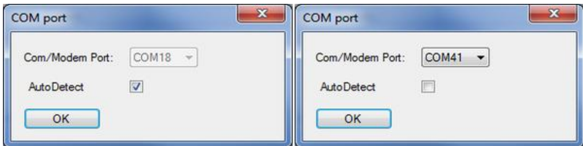
Fig. 5.5: Manually selecting the virtual COM Port of the Bluetooth or serial interface.
