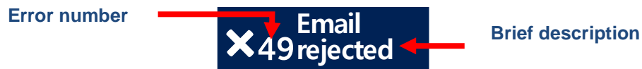
Fig. 6.5: Example of an error message appearing in the display. It includes the number of the error and a brief description.
