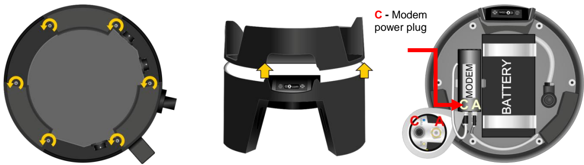
Fig. 4.4: Opening the X-zone Com housing (C = power plug, A = antenna socket).
